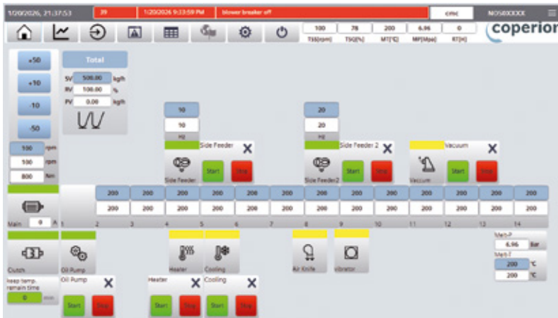
→ PLC human-machine interface of the STS twin screw extruder
