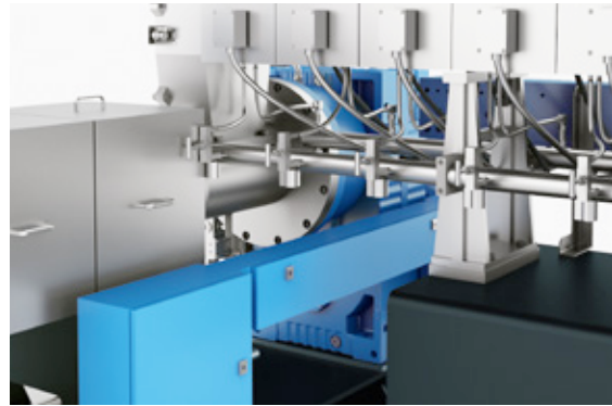
→ Transfer from twin screw to single screw process section
